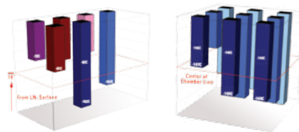
Comparison of temperature distribution in a liquid nitrogen freezer (vapor phase) and Panasonic's MDF-C2156VANC mechanically refrigerated cryogenic freezer. Graph shows temperatures at different locations within the chamber. This data demonstrates that 100% of the MDF-C2156VANC storage space maintains uniform storage temperatures safely below -130°C, while temperature in LN 2 vapor system is dependent on storage location.
