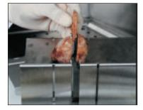
Raise the upper jaws and remove your 2 mm section from between the saw blades. The entire unit disassembles without tools for easy cleaning or disinfection.
