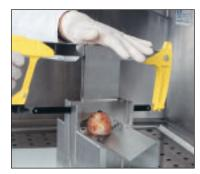
Raise the upper jaws and remove your 2 mm section from between the saw blades. The entire unit disassembles without tools for easy cleaning or disinfection.
