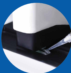
Load Cell Suspension into Sample Chamber
