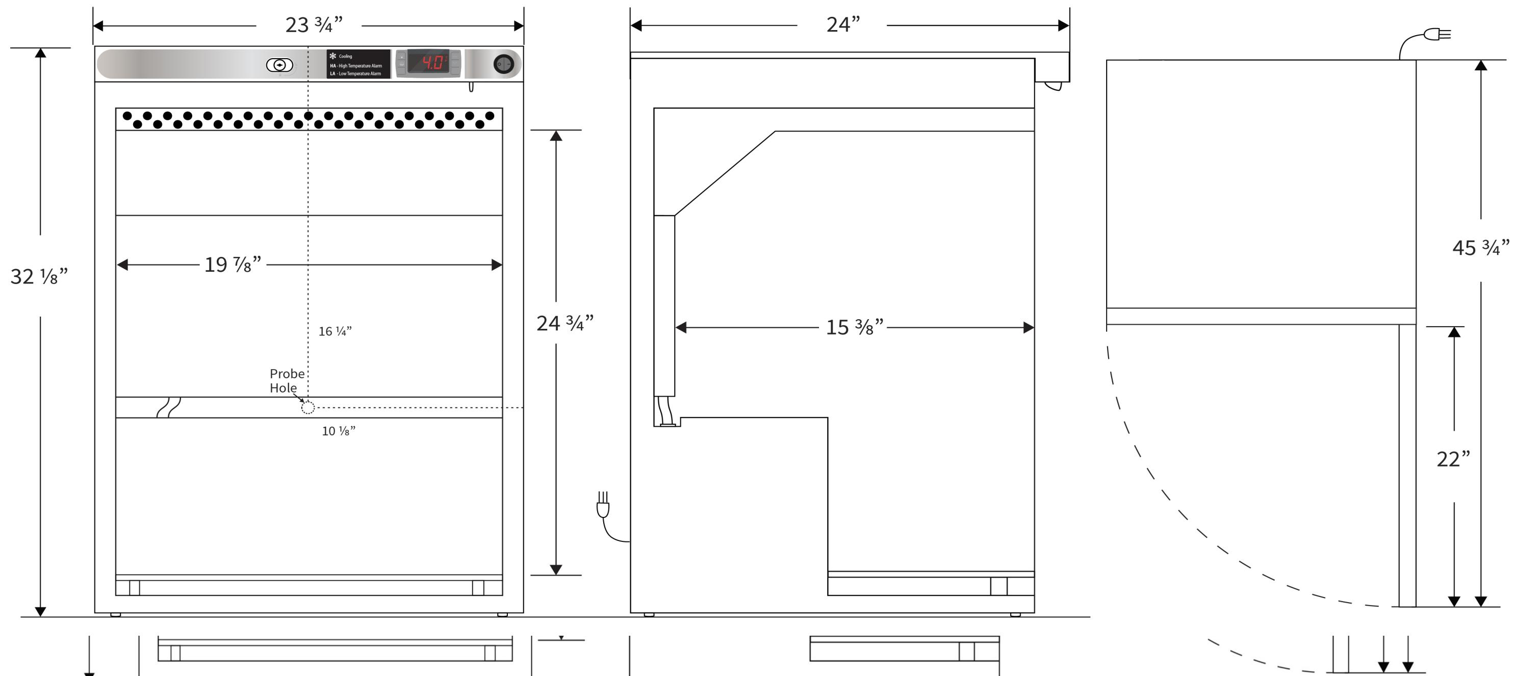
Note: This unit must have 4" clearance on sides and back for adequate ventilation
