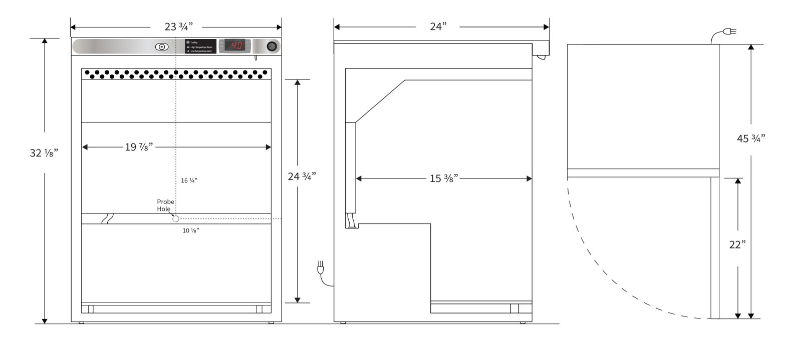
Note: This unit must have 4" clearance on sides and back for adequate ventilation
