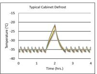
Performance data acquired at 22°C ambient, 4°C nominal set point in an empty cabinet with drawers using air probes, during stabilized steady state operation and a DAQ sampling rate of one measurement every 10 seconds
