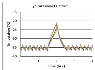
Performance data acquired at 22°C ambient, -35°C nominal set point in an empty cabinet with shelves using air probes, during stabilized steady state operation and a DAQ sampling rate of one measurement every 10 seconds
