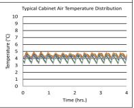
Performance data acquired at 22°C ambient, 4°C nominal set point in an empty cabinet with drawers using air probes, during stabilized steady state operation and a DAQ sampling rate of one measurement every 10 seconds
