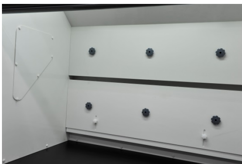
Legacy Standard Bypass and Baffle System
