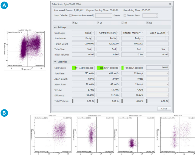
Mixed Mode Sorting. CytoTROL Control Cells (Part Number 6604248) were stained with DURAClone IM T Cell Subsets Antibody Panel (Part Number B53328). A four-way sort was set up to isolate Naive, Central Memory, Effector Memory, and aborts from all three sort streams, panel A. The resulting sorted populations were re-analyzed, panel B. CD197 (CCR7)-PE staining shows loss of signal post sorting, as expected due to photobleaching of this fluorochrome. All plots were gated for CD3+CD4+ singlet lymphocytes.
