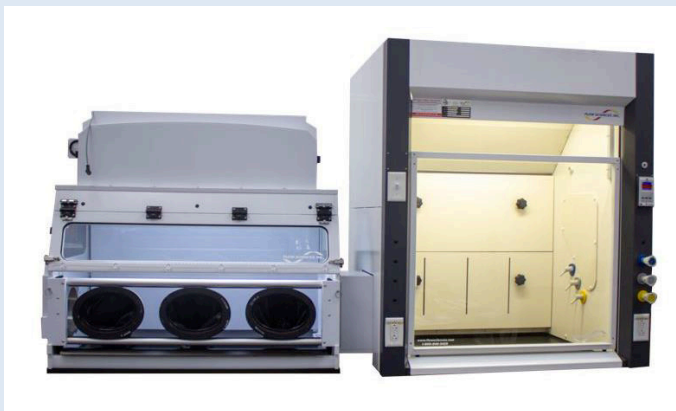
Fume hood connected to a lateral flow glovebox for continuous process work.
