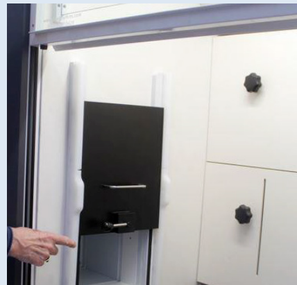
Fume hood connected to a lateral flow glovebox for continuous process work.
