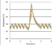
Notes an Performance Data: Performance data acquired at 22°C ambient, 5°C/-33°C naminal set points in an empty cabinet with shelves using air probes, during stabilized steady state operation and a DAQ sampling rate of one measurement every 10 seconds
