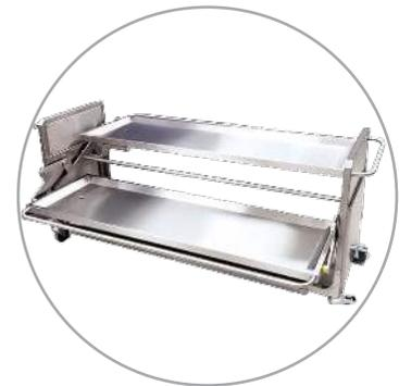
**Note:** The HM100 should be loaded, unloaded, and trays rotated by two operators to ensure a smooth and safe rotation. The cart is operated by manual force of pulling the bottom tray toward the operator and up. The weight of the cadavers must be within approximately 20 pounds of each other. Any overtly imbalanced load may make it difficult to rotate the trays.
