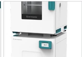
Two-unit stacking for improved space efficiency (option)
